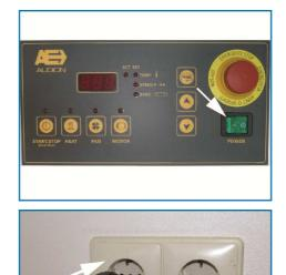
2. Insert the plug in the wall socket.
