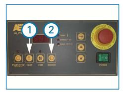
The heating and the transport motor must always be switched on before use.
