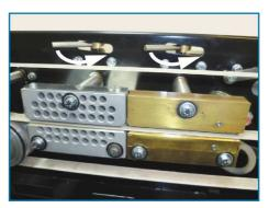
Pull the lifting pin up and turn the lifting plate so that the lifting pin can go back down all the way again.
