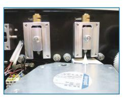
Try to keep the contact force as low as possible in order to minimise wear and tear on the PTFE belts.
